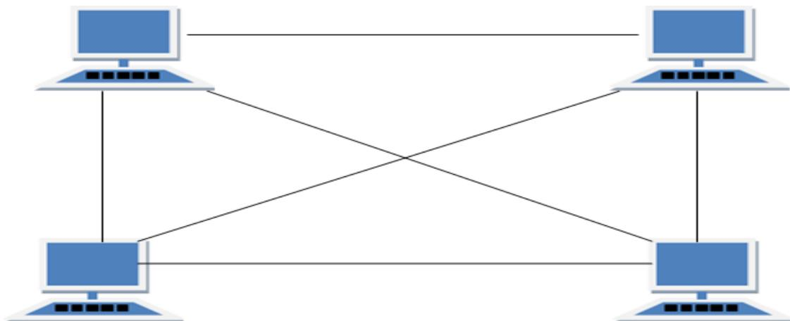
Mesh topology is a group of nodes which are all connected to each other and many types of connections are possible in a mesh topology.
