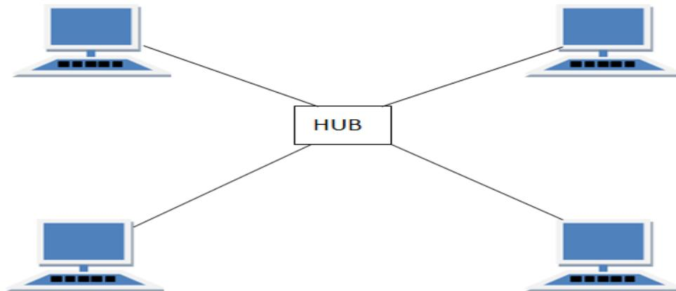
A STAR topology is based on a central node which acts as a hub. In star topology each node is directly connected to a Hub/Switch.
