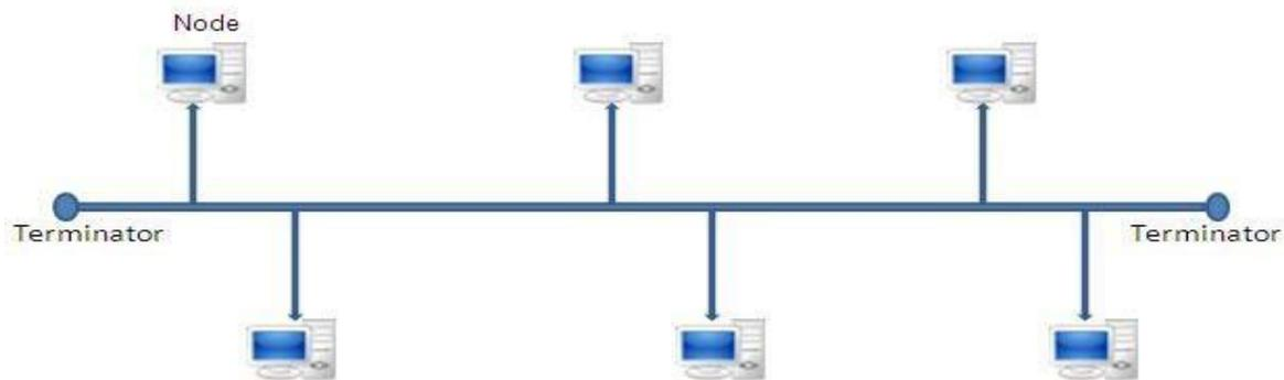
**Bus Topology** :-Bus topology is a topology for a Local Area Network (LAN) in which all the nodes are connected to a single cable. The starting and ending point of cable is called terminator.
